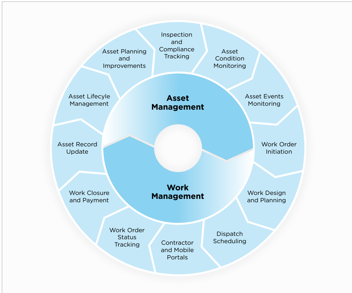
Figure 1: Lifecycle of asset and work data
